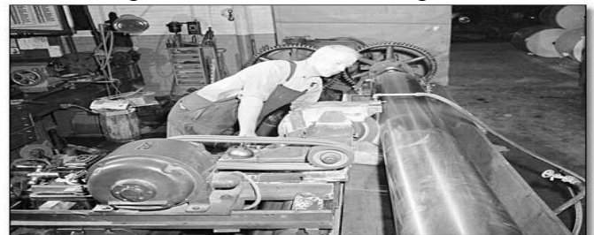
Nick using Tom's older lathe to make some axle bushings for Adam. Nick set up the lathe for Adam and Andy helped. Tm
