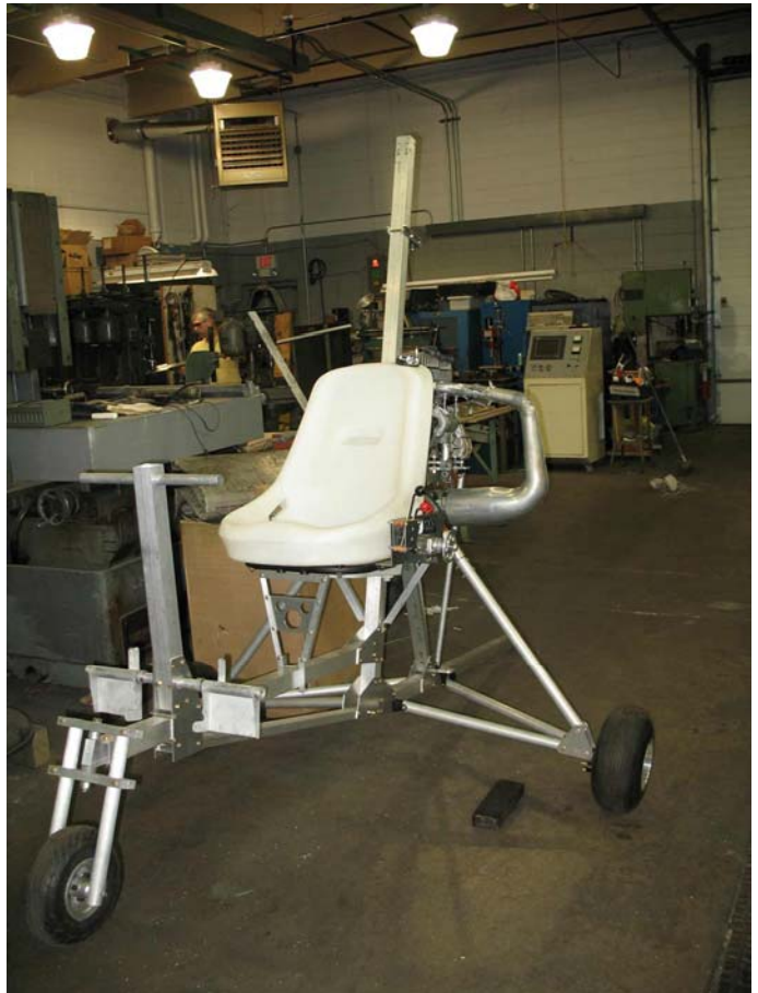
Adam's Monster Gyro, as of June 27 th . Recent updates include muffler, throttle quadrant, and pedals.
