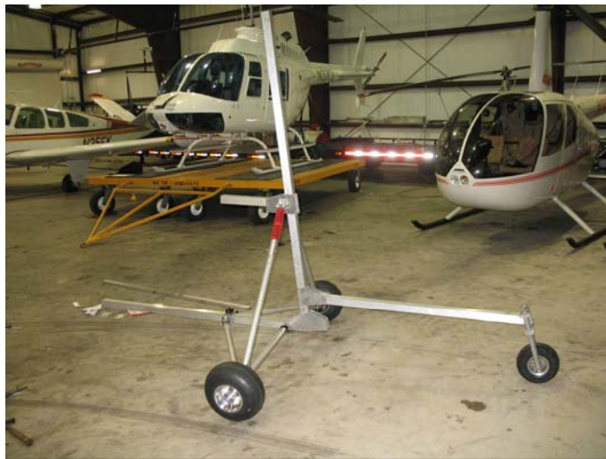
Adam's airframe, complete with shocks and all. The frame itself went together without a hitch, but it's the little things that are causing some holdups with assembly. We have moved the machine to ABET to speed some things up.
