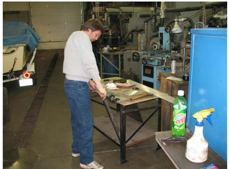
Randy Myers transfers cluster plate outlines and holes onto a sheet of aluminum.
