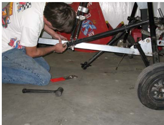
Randy Meyers works on reassembling his gyro after making a new rear keel.
